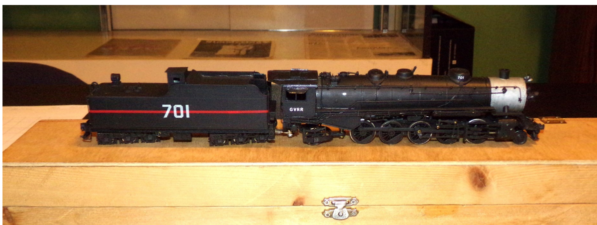
Anthony Parrish: A Bowser Locomotive Kit with brass tender, modified fire box, and cab. He added all the details to locomotive and added dog house and backup lamp to tender.
