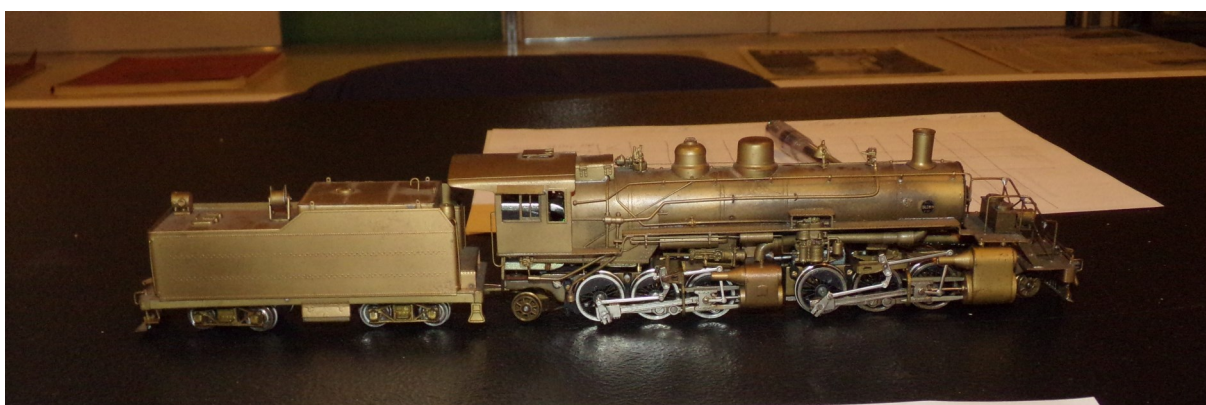
Mark Maynard: Very old unpainted brass Pacific Fast Mail 2-6-6-2. These types of older brass locomotives are becoming very popular as candidates for motor upgrades and DCC conversion.
